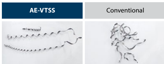
Chip shape from plunging
